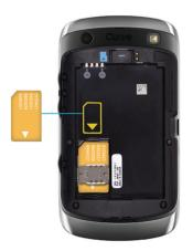
Slide the SIM card into the slot.
